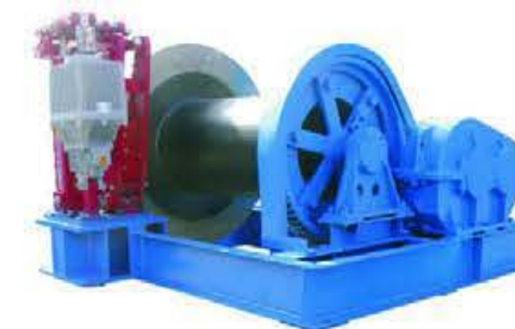
JM10T Low speed winch, pull capacity 100KN Rope speed:9.5m/min rope capacity 300m Used for 80T gantry crane in China Railway Bridge Bureau
