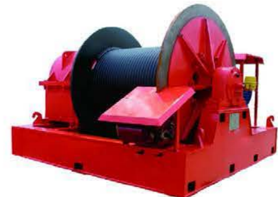
JM12T Low speed winch used for 900T overhead crane in China Railway 14th Bureau Rope speed: 14m/min rope capacity 410 m
