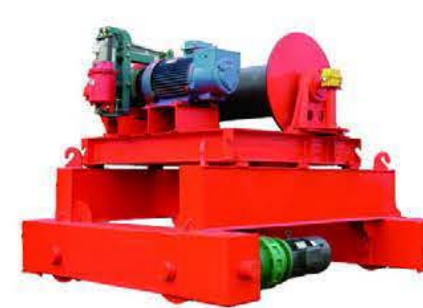
JC80T Engineering door crane trolley Lift capacity:80T Lift speed:0.8m/min Lift height:21m Rail gauge:2.5m
